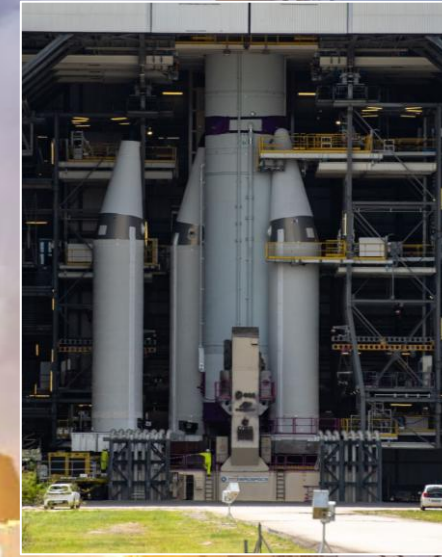
Installation of 4 P160C boosters on central core
