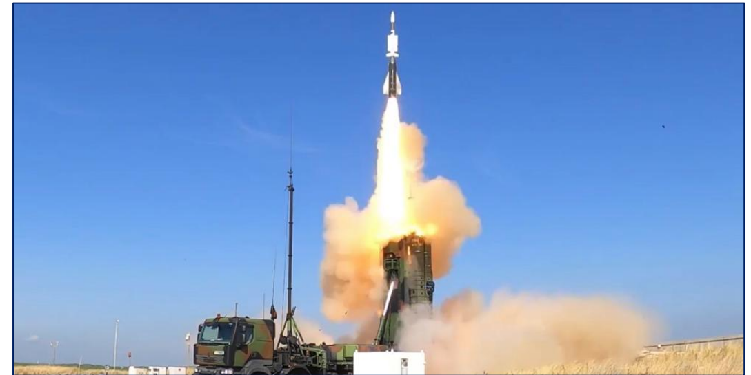
Launcher module of a SAMP/T NG air defense system
