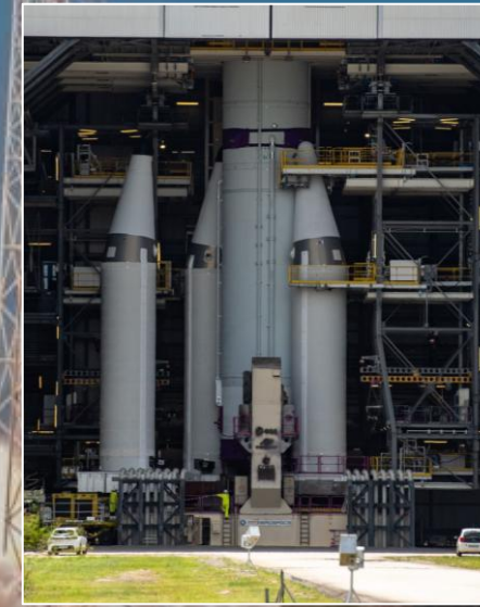
Installation of 4 P160C boosters on central core
