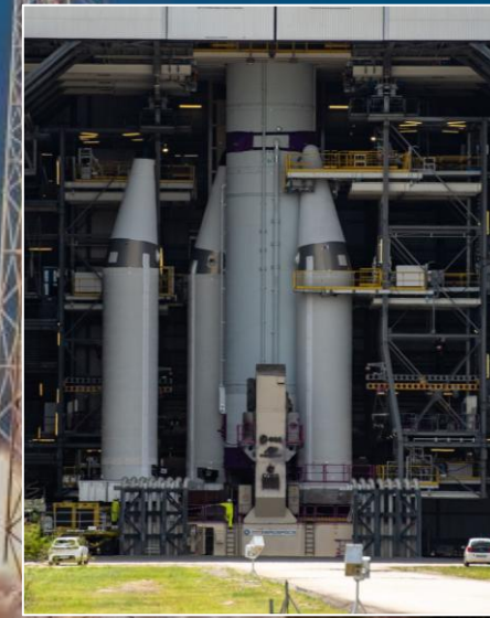
Installation of 4 P160C boosters on central core
