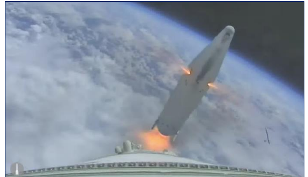
P120 booster separation
