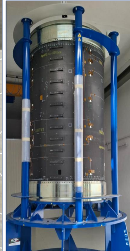
Cryotank static load test
