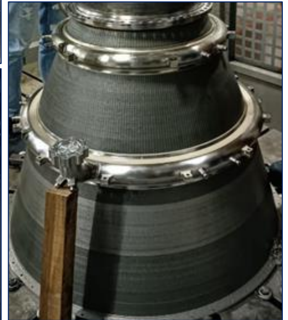
MR10 regenerative-cooled nozzle extension
