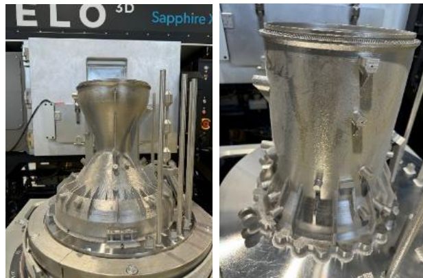
M10 for IFD1 Flight: manufacturing on going, TCA and Nozzle Printed in house
