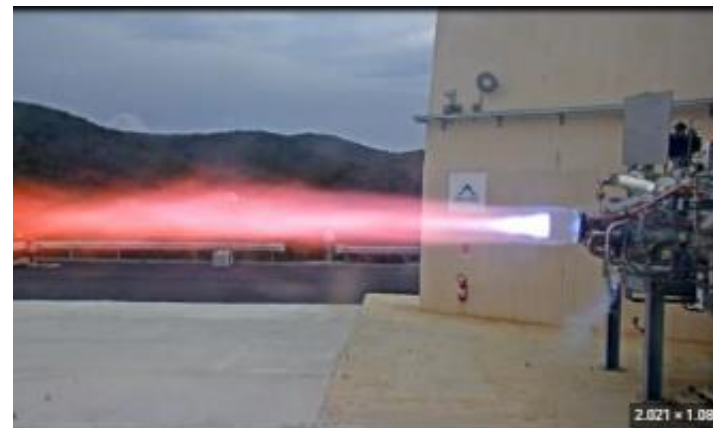
DM1 (2022) and DM2 (2023) M10 Engine Firing Tests
