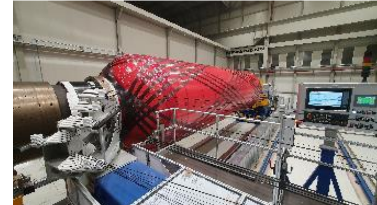
IMC, Composite case during winding (initial phase)
