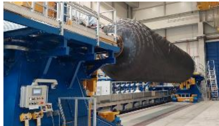
IMC, Composite Case winding
