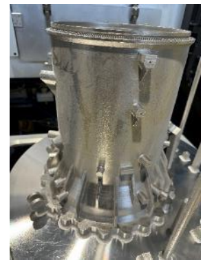
M10 for IFD1 Flight: manufacturing on going, TCA and Nozzle Printed in house
