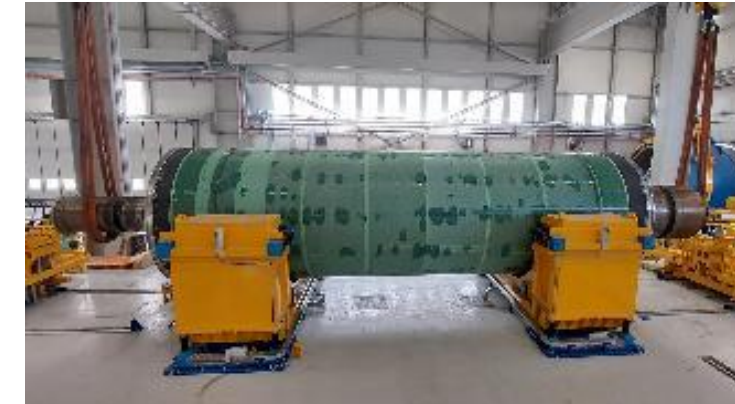
IMC, Composite case after thermal curing
