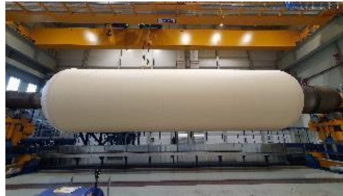
IMC, Thermal Protection after machining
