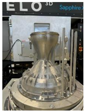
M10 for IFD1 Flight: manufacturing on going, TCA and Nozzle Printed in house
