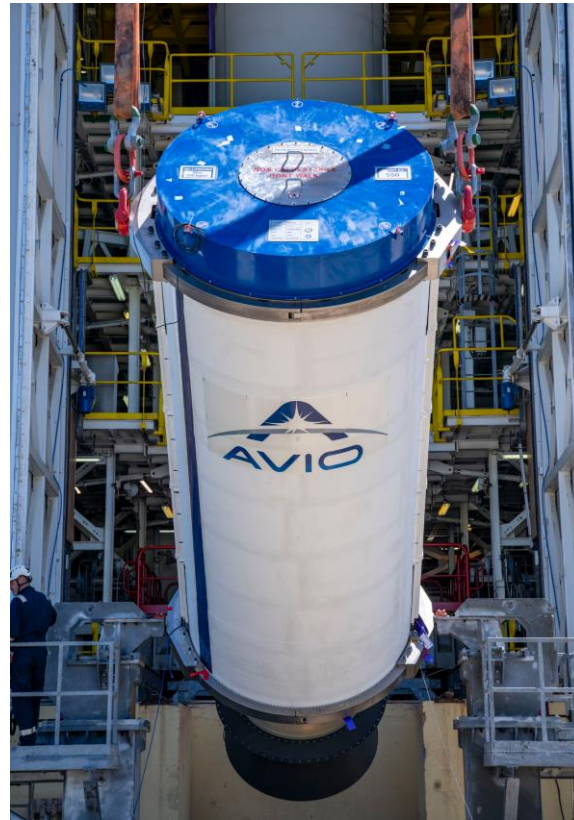
Hoisting Zefiro-40 stage
