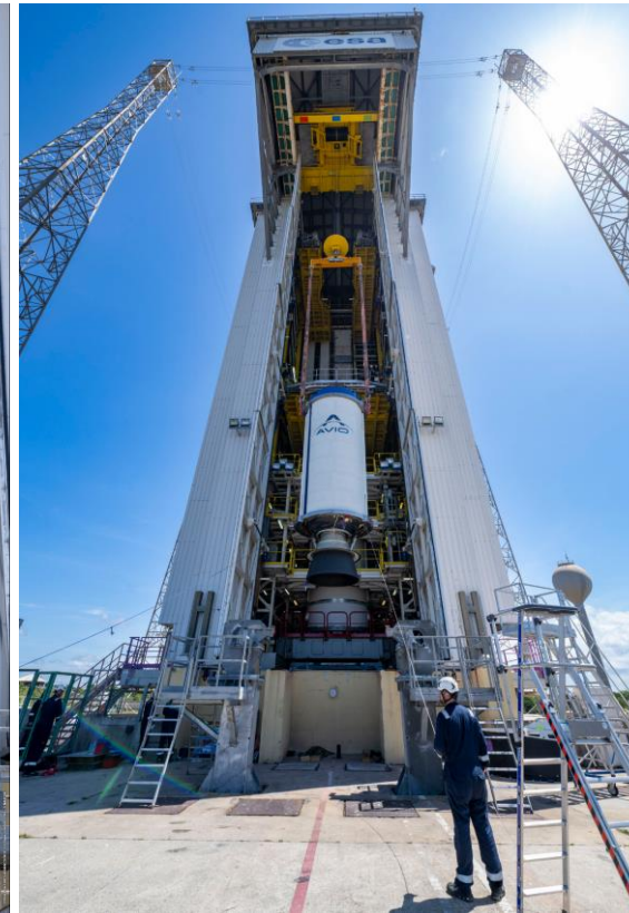
Hoisting Zefiro-40 stage
