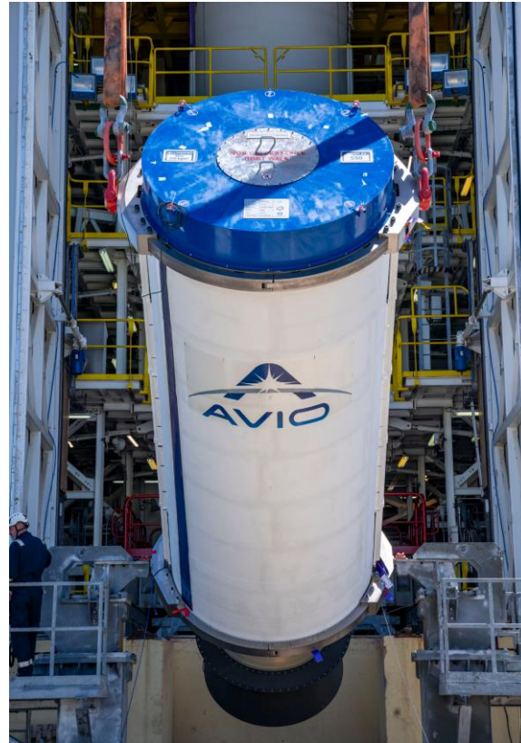
Hoisting Zefiro-40 stage
