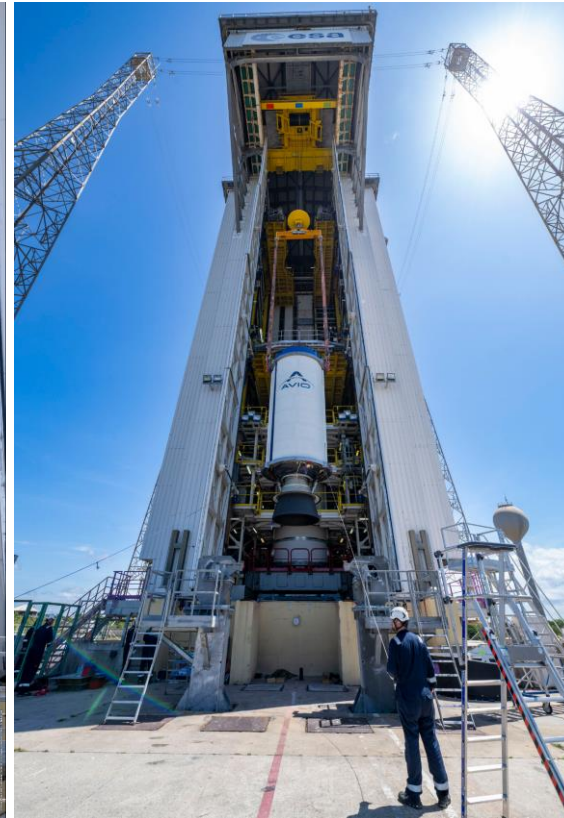
Hoisting Zefiro-40 stage
