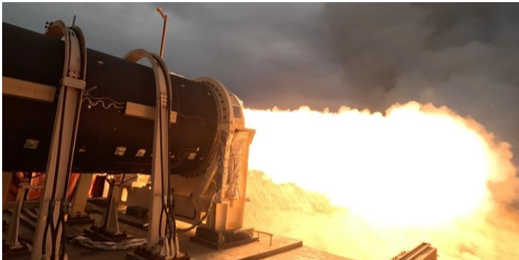
SRM testing (P120 and Z40)
