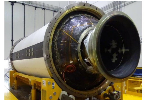
Z40 engine getting ready for the static firing test
