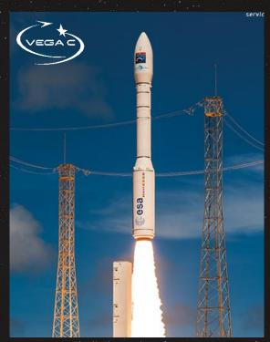
European light launcher (2.3 tons in LEO) **Avio: System integrator**
