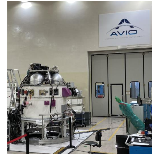
A4 upper stage avionics, environmental and fluidic testing in progress in Colleferro
