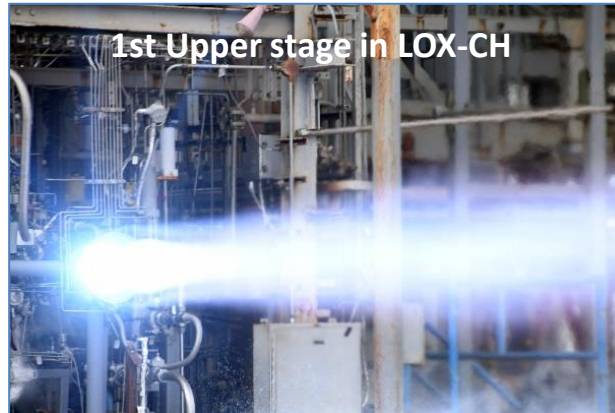
Vega E: M10 LOX-CH firing test (USA)
