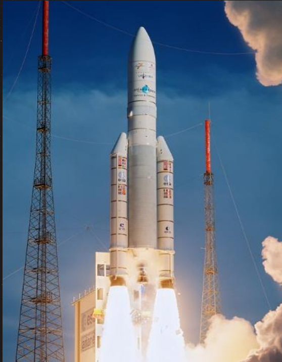
European heavy launcher (10.5 tons in GTO) Avio: Strap-on boosters
