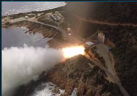
Vega C: Zefiro40 firing test (Sardinia)
