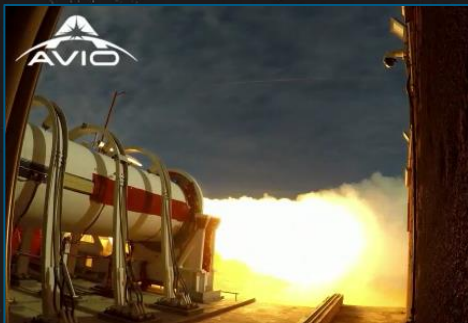
Return to flight: Zefiro23 firing test (Sardinia)
