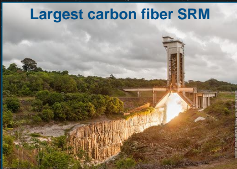
A6/Vega C: P120 firing test (Kourou)
