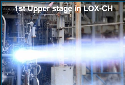
Vega E: M10 LOX-CH firing test (USA)
