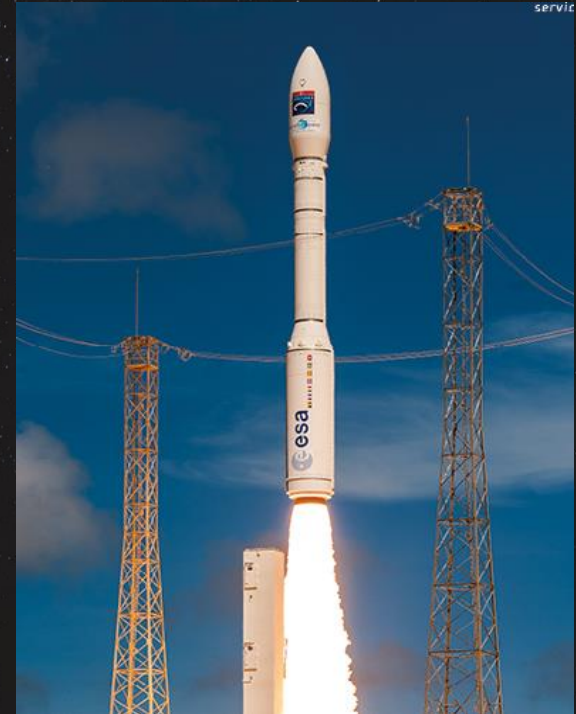
European light launcher (1.5 tons in LEO) Avio: System integrator
