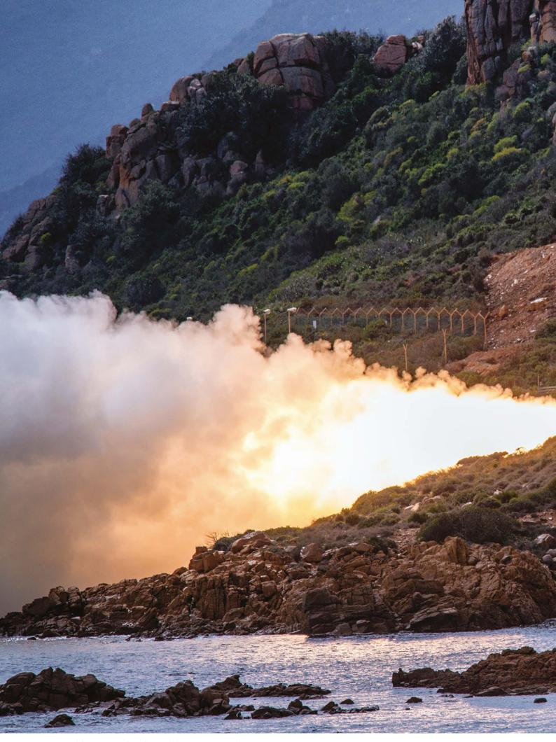
Firing test of the Z23 engine from the Salto di Quirra range in Sardinia
