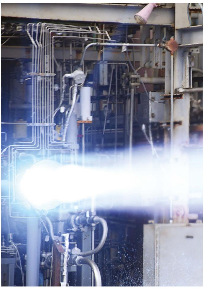
Motor M10 firing test, last stage VEGA E
