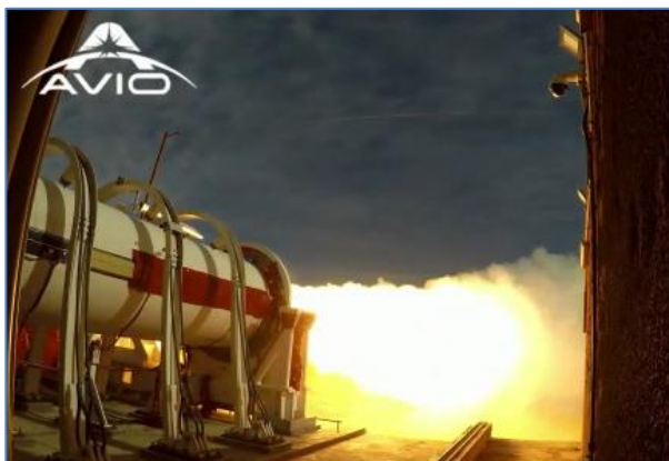
Return to flight: Zefiro23 firing test (Sardinia)
