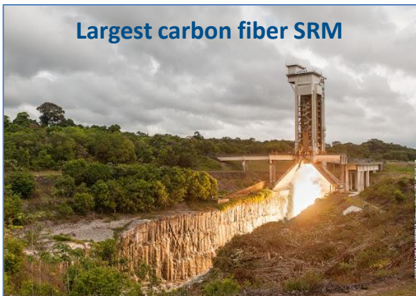
A6/Vega C: P120 firing test (Kourou)
