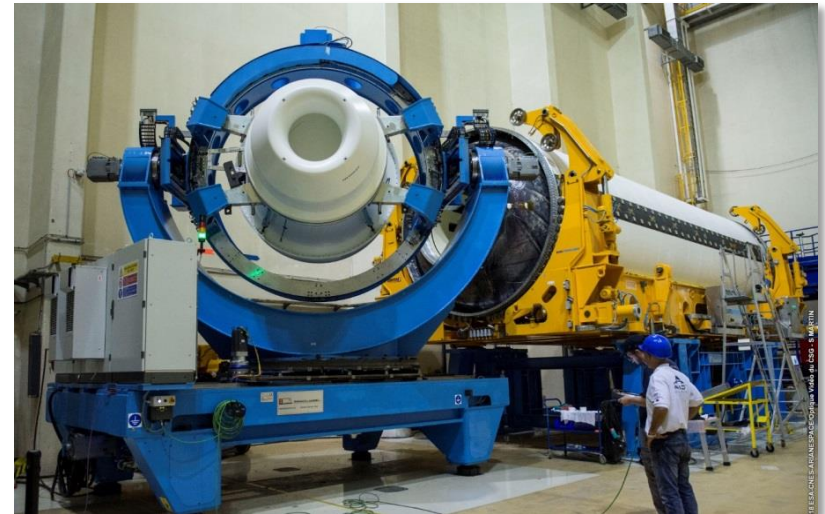
Automated nozzle integration (Europropulsion)
