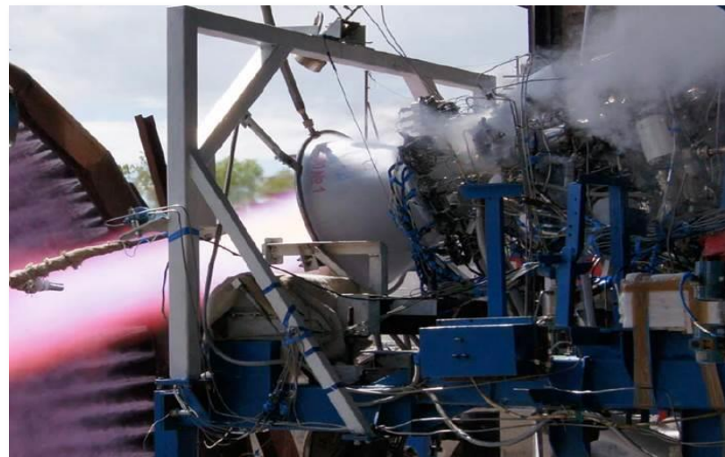
MIRA upper stage engine firing test
