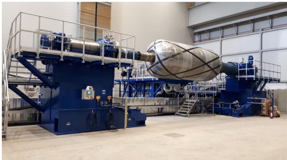
New filament winding and automatic tape layup machine
