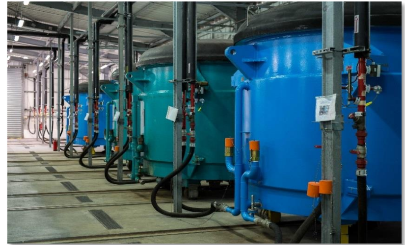
New Vega C propellant casting pots (Regulus)
