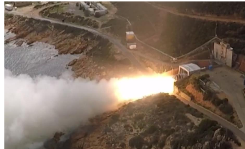
Z40 Static Firing Test
