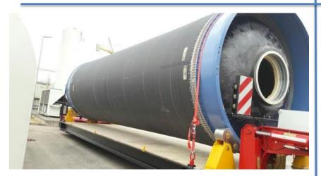
P120 IMC\* completed (world's largest carbon fibre monolithic solid rocket motor case – 142ton)
