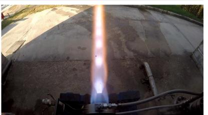
Successful LOx-CH combustion chamber test for upper stage engine
