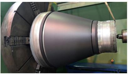
Z40 nozzle carbon-phenolic exit cone manufactured
