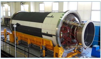
Fully integrated Z40 and ready for firing test
