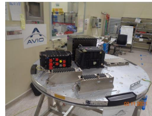
A4 upper stage flight item under integration
