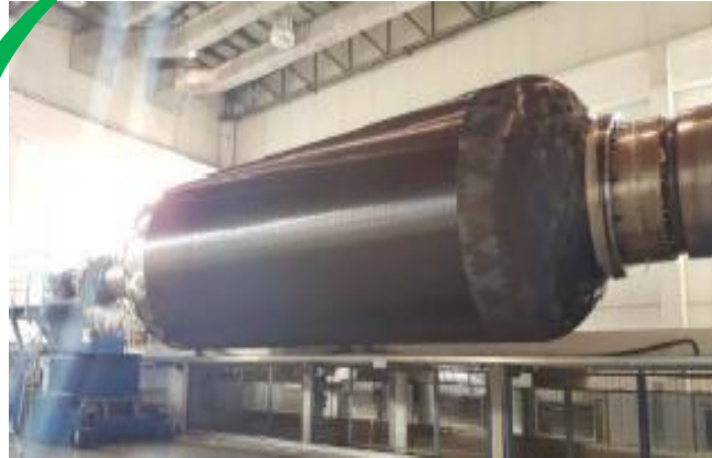
Z23 Filament winding completion
